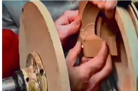
Pressing the dowels into the predrilled holes for final alignment.
