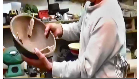
Before going to the bandsaw, a series of blocks are hot-glued inside.
