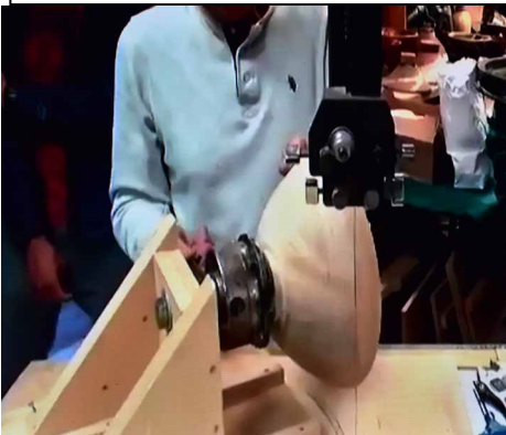
Making the first cut by swinging the fixture against the bandsaw.
