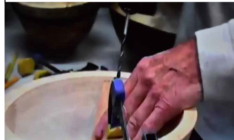
Holes are drilled through each block. Dowels are inserted into the holes for fit and removed before going to the bandsaw.
