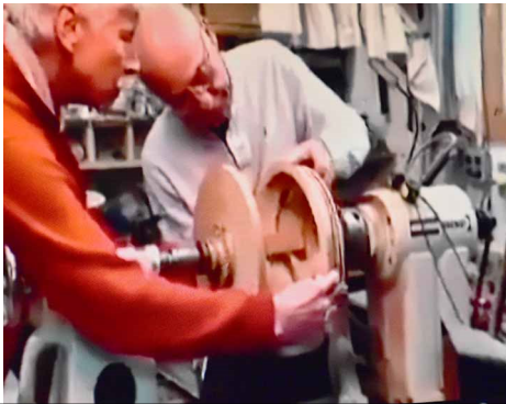
Assembling the complete bowl blank on the lathe. Glue is applied during this step.
