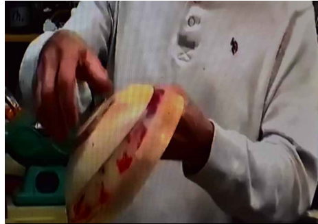
Another example. The wave section has epoxy fill-ins.
