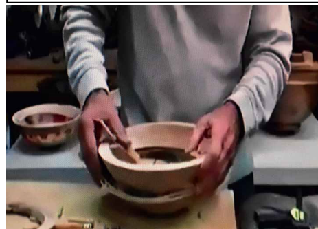
Placing the top of the bowl on the bottom assembly for fit.
