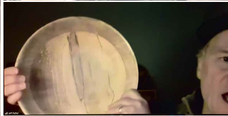
Jeff Petter showed some spalted maple pieces he's working on, experimenting with various finishes. Mickey Palmer recommends Parfix 3408 CA glue to stabilize soft woods.
