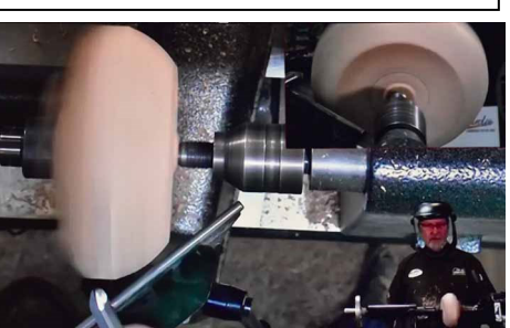
Beginning to shape the exterior using a 45 degree bowl gouge.
