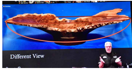
A burl can be turned from the top (left) or the bottom (right)
