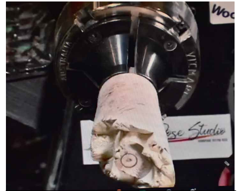
Now to start hollowing into a cup shape, leaving enough character.
