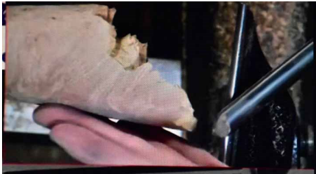
The initial hollowing can be made with a smaller, higher angle bowl gouge.
