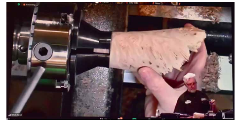
Reverse the blank into a scroll chuck.
