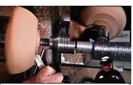
Shaping the tenon. This scraper gives a square shoulder.
