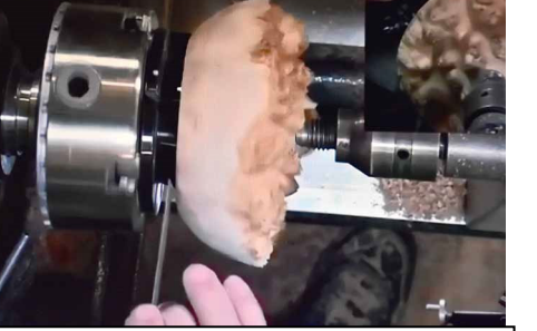
The piece is turned around and mounted squarely into a scroll chuck.
