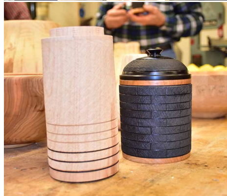
Ted uses a grinder to apply texture to his boxes. Takes a few seconds. He also uses a "veiner" and a wire to make grooves and burn them in. Shoe polish provides the color.
