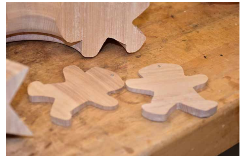
Dave used the German "ring" method to make both star and gingerbread man ornaments. Turn a ring in the right shape, then cut off slices with a band-saw.
