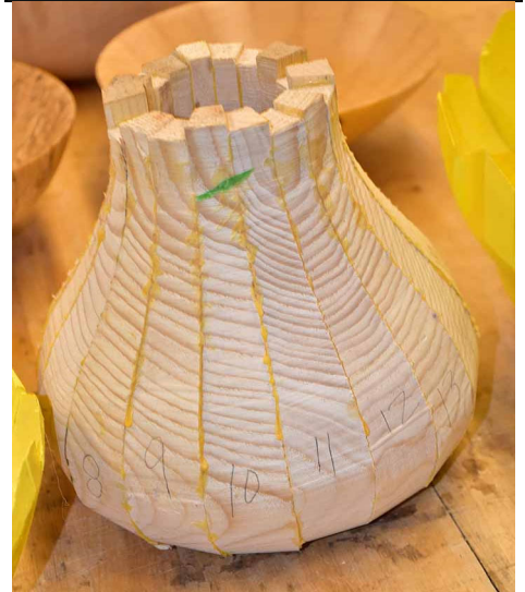
This unit is glued but not yet turned to final shape.
