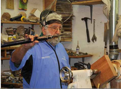
Starting with a gouge, Al prepares the bottom of a workpiece.
