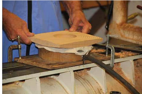
The bowl is mounted and the vacuum attached & turned on.
