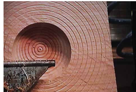
Back on the lathe to scribe concentric circles on the face.
