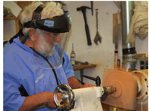
The plate is reversed and the front is started.
