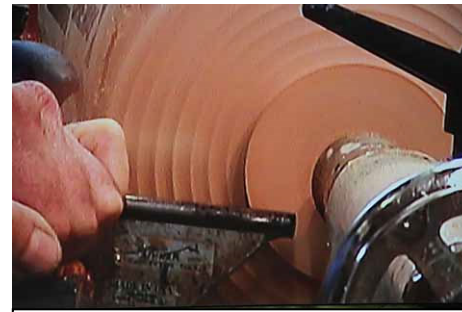
Nice, even grooves are formed on the back.
