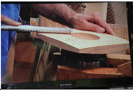
Using a rasp to roughen the face.
