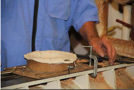
Now, Al uses a vacuum fixture to hold the bowl for more carving.
