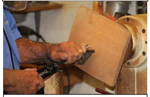
Reversed again & the tenon removed.
