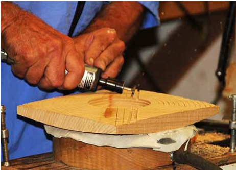
Here, he is etching lines into the face of the bowl.
