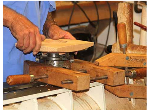
The chuck is used as a carving stand.
