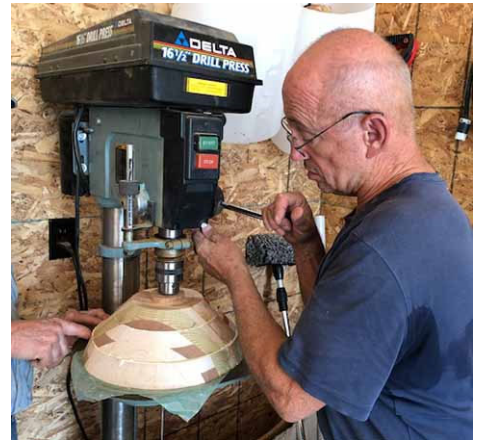
Ted using a drill press as a bowl press, a lathe could work too
