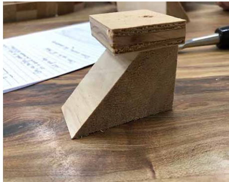
Handy jig for gluing ring halves together
