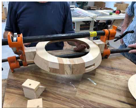
Jig in action with clamps
