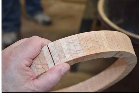
Some glues can “blush” and allow the joints to show off.
