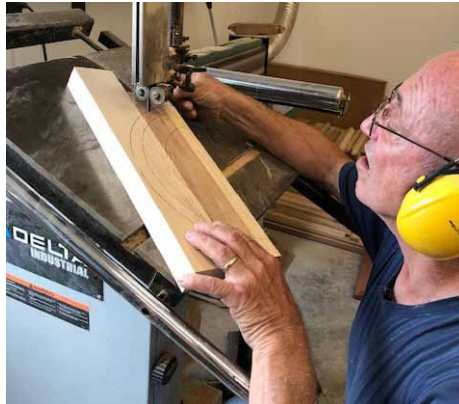
Cutting rings on the bandsaw set at an angle.
