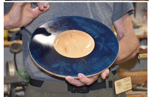
David is experimenting with a photographic process to transfer images onto platters. This process was used to make blueprints. The chemicals are still available.
