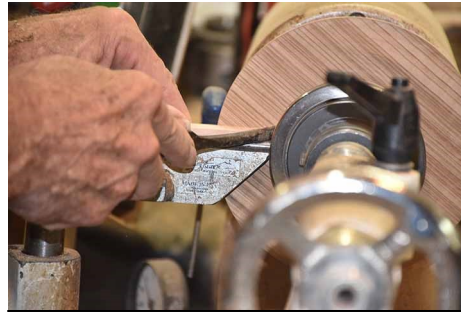
You can grind a screwdriver down to make the parting tool.
