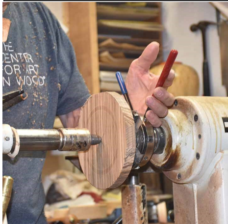
The object is rechucked using a 4-jaw.
