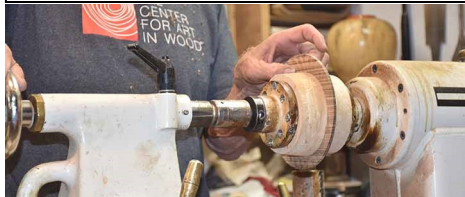
Two jam chucks to fit onto the inner ring are used next. If you want more rings, size another set.
