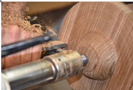
The next step is to start thinning down the "ring" part. Note that a tenon is left on the bottom for rechucking and reversing on the lathe.
