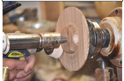
The "rings" are thinned down, leaving a center part raised. Its diameter should be the same as the bowl part on the bottom.
