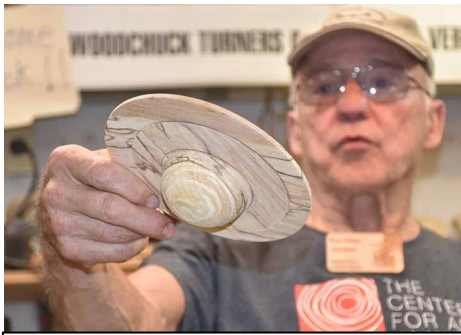
A Saturn bowl uses offset turning, many jam chucks, some special tools, and great steadiness.
