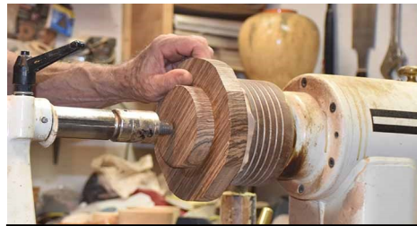
We start by gluing up the rough shape; a bowl section glued to a ring section.
