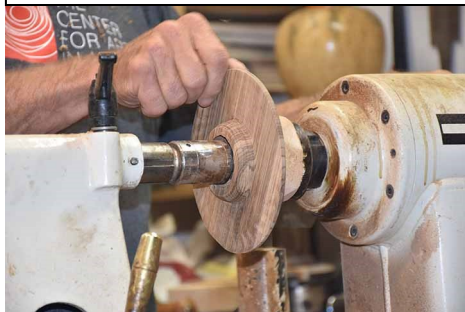
Using a jam chuck and a live tailstock, the piece is re mounted in preparation for parting off the rings.
