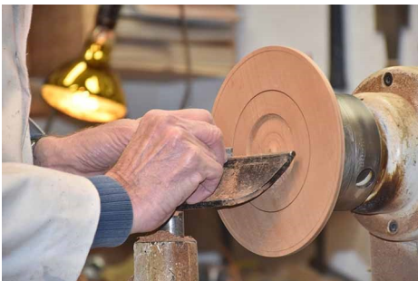
Dave uses a narrow parting tool to scribe borders. He then uses a scrap of Formica to burn the inscribed border lines.
