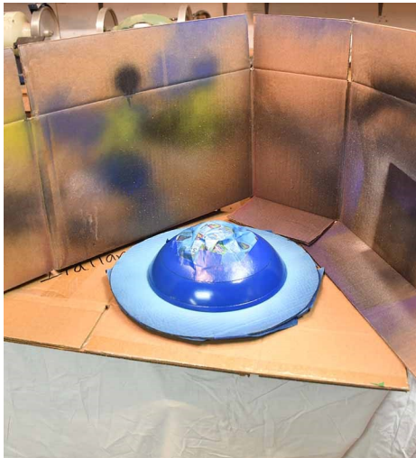
After masking, the object is sprayed with the base color and allowed to thoroughly dry.
