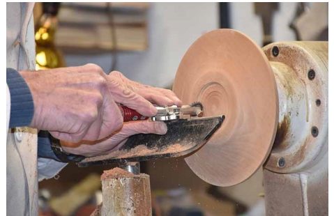
He uses an inset about 3/16" deep to fit the expansion jaws of a chuck.
