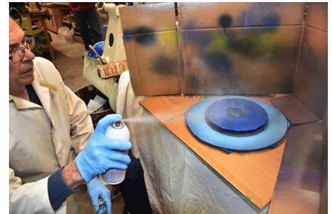
A can of acrylic is then sprayed at a low angle across the object. White is being used for the first color.
