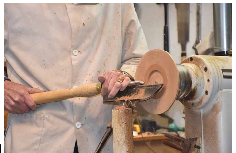
Dave then turns the blank over, re-attaches it to the lathe then forms the bowl area. He finishes the hollowing out after the spray-on decorating is finished.
