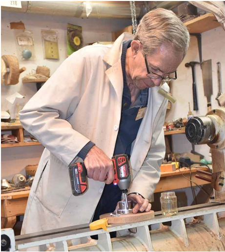
Dave starts by screwing a platter blank to a faceplate, using Spax coarse screws..
