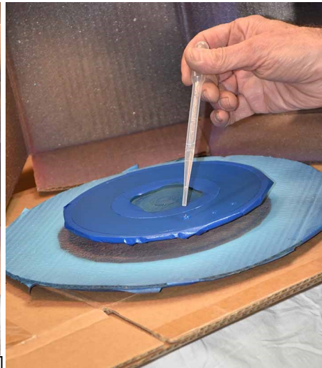
Water is dripped onto the object. Use a fine spray for smaller droplets.
