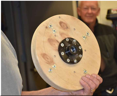
The next step was to construct a large faceplate specifically for the retainer rings. It has a double thickness of 3/4 inch plywood with T-nuts on the reverse to take through-bolts.
