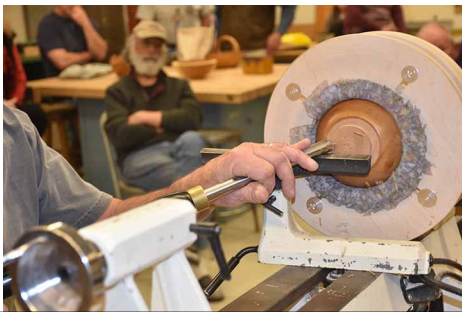
The tenon is then turned off, and the base finished with a recessed groove before final sanding and finishing.
