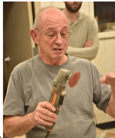
Ted modified a Job Max to use 2" round hook & loop pads to fine sand parts of his work.
