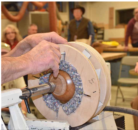
The retaining ring is then fastened to the faceplate using 4 bolts & washers; carefully centered, and tightened enough to firmly hold the bowl in place.
