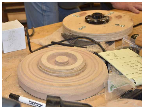
Ted tried using jam chucks to hold bowls for tenon removal, but the variety of sizes started to waste time and wood.
