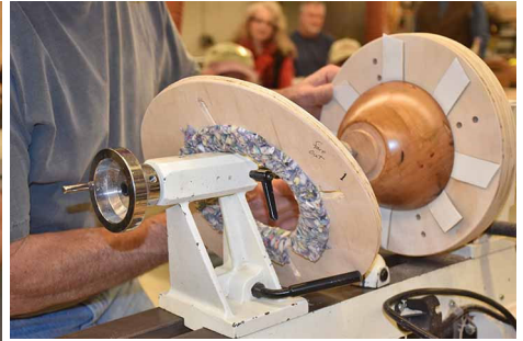
Each bowl is carefully centered using the tailstock holding in a dimple on the tenon.
