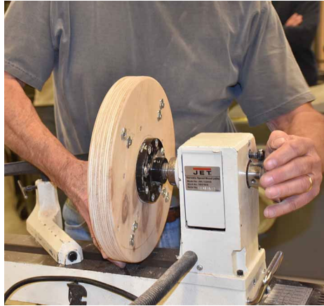
The faceplate was trued up and then drilled to accurately hold bowls centered.
