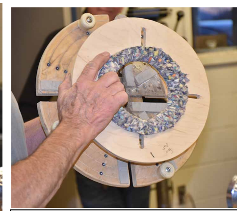
The next step was to make a hold down ring and clamp bowls that way. The modified Cole jaws still offered some accuracy problems.
