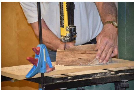
Here is a jig for preparing blanks on a bandsaw. It uses a pin to center the blank.
