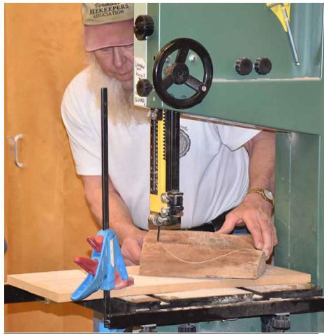
By clamping the jig to the table, the jig can be tilted and conical blanks can be taken out.
