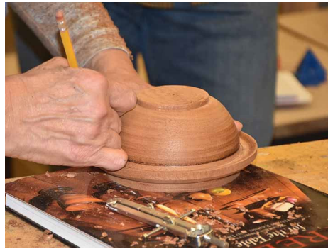
She's scribing the handles. The handles should be with the grain, not across, for strength.
