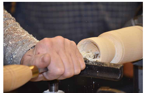
The outside of the cup is refined and the inside is thinned down to final thickness.
