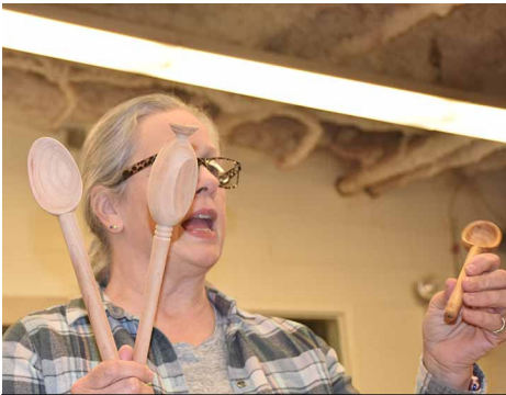
Wooden spoons of many sizes and types are possible on the lathe. Much of the form can be turned (right) then the bowl carved using hooks or gouges.
