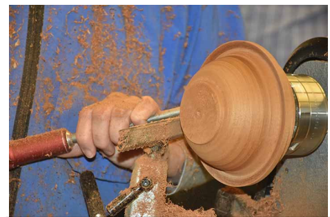
Here, she has the outside bowl shape nearly defined, the foot taking shape, and is working to undercut on the underside of what will be the handles
