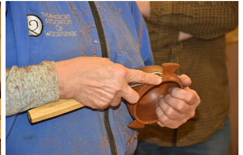
The waste has been band sawn. The rim has been sanded and textured. She's now using a carving tool to refine the curve on the handles.
