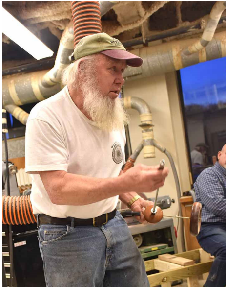
Bob's device for turning the end of a dowel. It goes right through the headstock and is drawn tight by the wooden handwheel.
