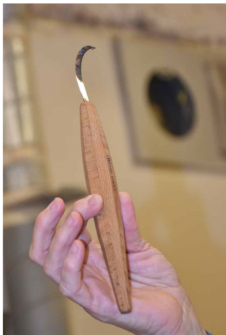
This delicate tool is a hook used for carving out small vessels.
