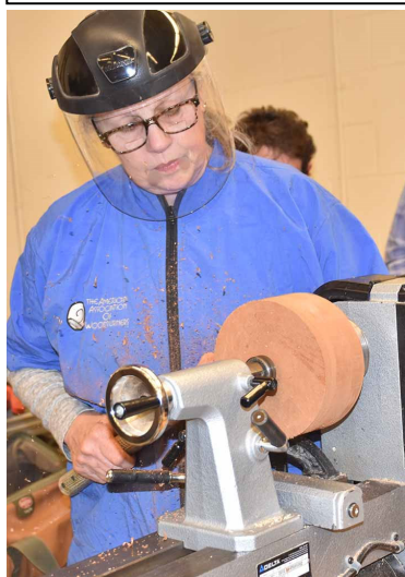
For a porringer, Janet mounts up a round of mahogany and forms a tenon.
