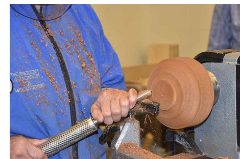
Remounting it, she quickly forms the outside, making a base and starting the double rim.
