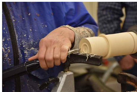
A tenon has been cut. The blank has been portioned; cup, stem, & base. The cup starts to be formed and hollowed.
