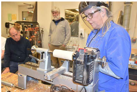
OK. Let's start on a goblet. A billet is mounted between centers and rough turned. Grain is parallel to the bed.
