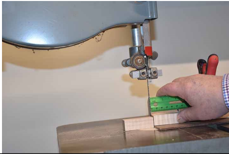
Step 1 is to cut the blanks to size. I made a sled to measure and cut on my band-saw.
