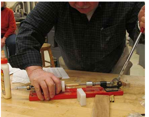
Finally the parts are assembled with the aid of a pen press.
