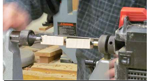
The blanks are then mounted alternating with the bushings on the mandrel. The mandrel is mounted on the lathe and the tailstock is brought up with enough pressure to get the blanks spinning when the gouge is brought to bear. As the diameter of the blanks is below an inch, lathe speed can be above 2000RPM.
