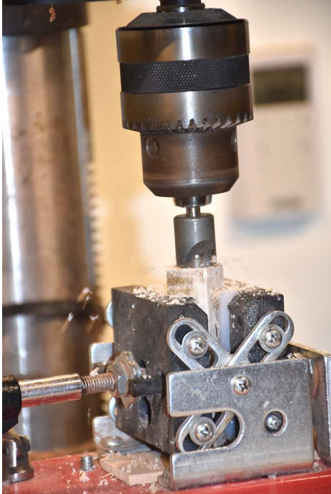
Both ends of each blank must be squared using the pen mill. Either the drill press with the vertical vise or the lathe can be used.
