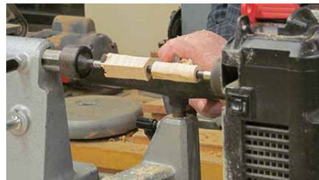
First, the roughing gouge is used to quickly take the blanks down to reasonable diameter.
