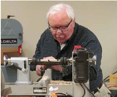
Then, either a spindle gouge or a skew gouge is used to bring the blanks down to final shape, with the ends very close to the same size as the bushings. The bushing diameter matches the diameter of the pen parts.
