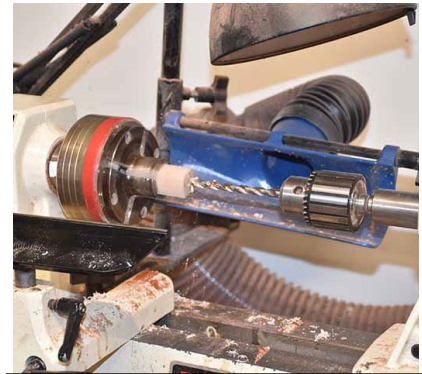
Step 2 is to drill the blanks. For these pens, a 7mm bit is used. In the drill press, a vertical vise is needed. On the lathe, a chuck with needle jaws and a Jacobs chuck holding the drill bit is efficient.
