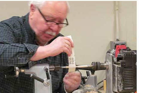
Sanding comes next. Several grades are used, ending up with 1500-grit.
