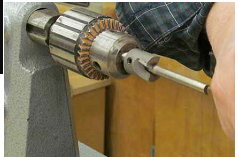
This is a pen mill in the Jacobs chuck used to square the blank with the end of the brass tube.
