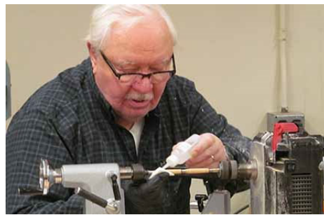
The CA glue is polished with an automobile compound.
