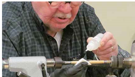
Several coats of thin CA glue are applied with a paper pad and hand protection.
