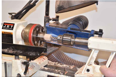
Both ends of each blank must be squared using the pen mill. Either the drill press with the vertical vise or the lathe can be used.
