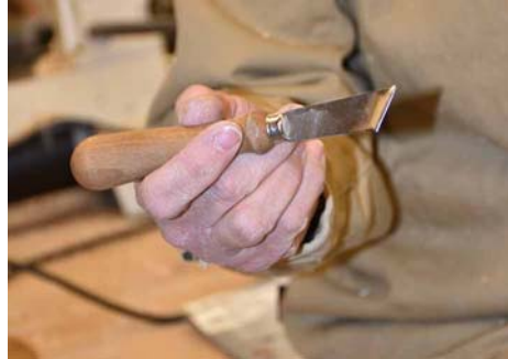
This is a chip carving knife—very sharp.
