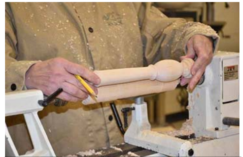
Using a pattern to mark off the divisions of the spoon shape.
