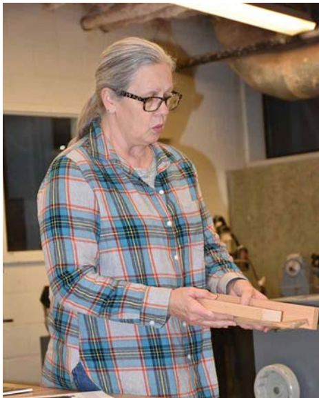
Start with 2 pieces of wood of equal dimensions. The thickness of each should be equal to 1/2 the width.
