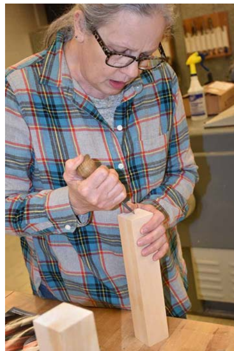
Use an awl or punch to mark the centers.
