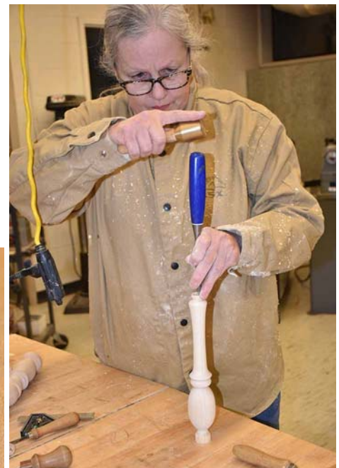
Using a chisel to split the 2 pieces.
