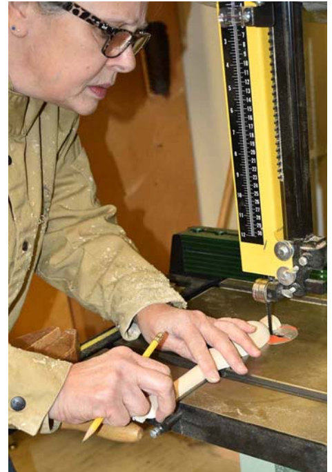
Saw off the waste from both ends of both pieces.
