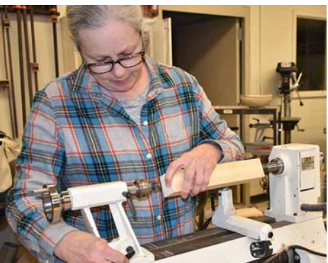
Using a cup live center mount the piece on the lathe. A Steb Center is a good choice for the drive end. The idea is to hold the wood without splitting the join.
