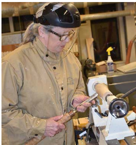
Using a cup live center mount the piece on the lathe. A Steb Center is a good choice for the drive end. The idea is to hold the wood without splitting the join.
