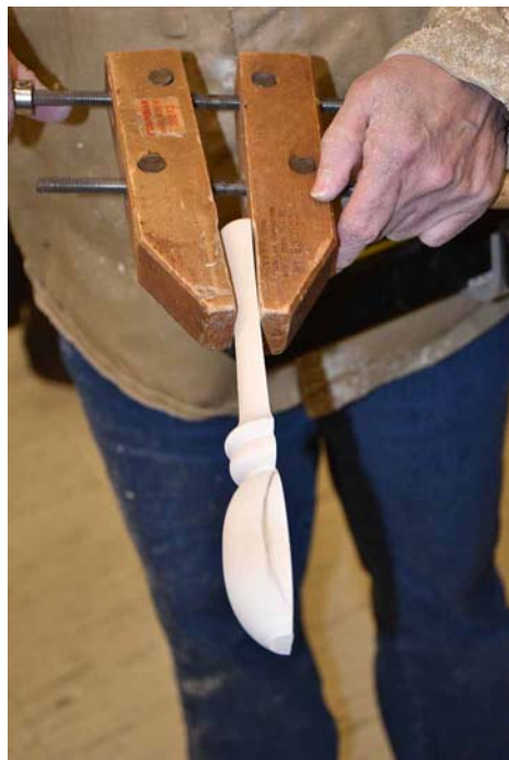
A wooden hand clamp is a safe way to hold the piece vertically for sawing the face of the bowl of the spoon.
