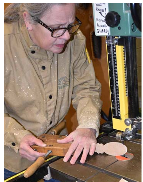
Cut the scoop shape with the bandsaw. The next step would be to use a burr or a spoon gouge to scoop out the bowl shape.
