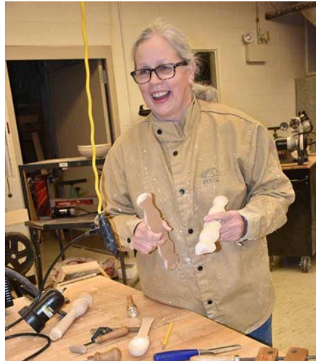
If your application of glue was even, the paper boundary gets split fairly evenly on both parts of the piece.
