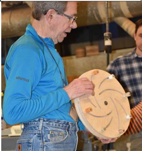
Dave found that artificial wine corks serve well on this shop-made platter holding rig.
