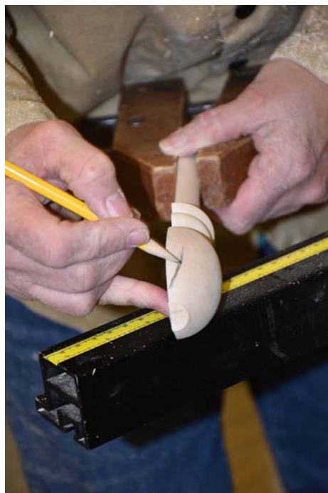
Draw a guide line for sawing the scoop shape.
