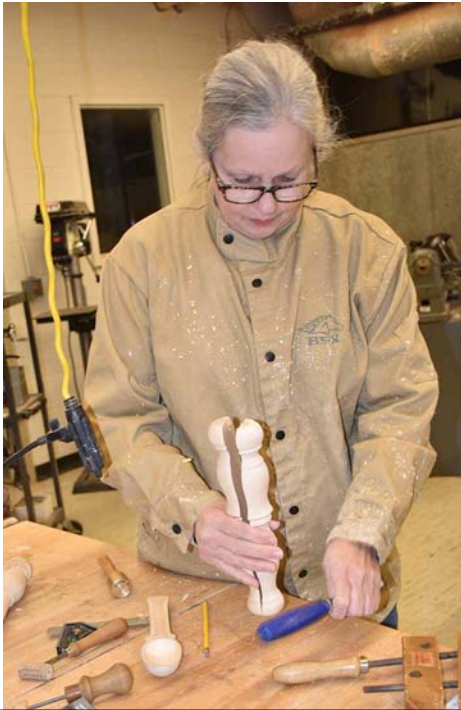
Work carefully from both ends of the piece with the chisel.
