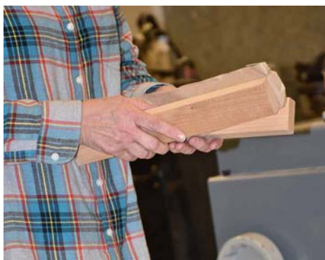
Use something like a paper bag as an interface. Glue the two pieces together with the paper between them. Titebond will do well. Let the glue dry before the next stage.
