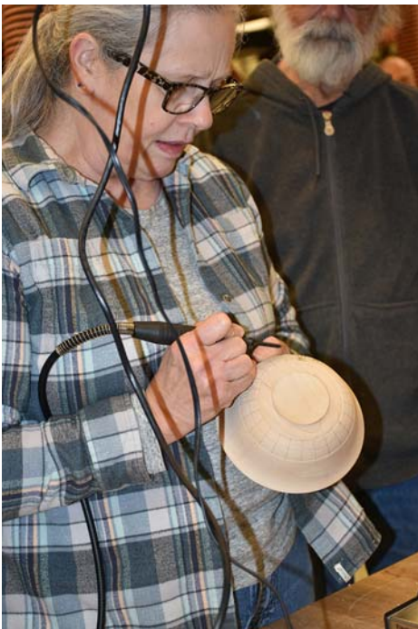
Dremel tools can be used with flex-shaft converters to make them impact carvers.
