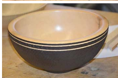
Ted showed a Cutsall grinder used to texture. By holding at a 45 degree angle, you can get an all-over pattern. The color is from black Krylon.
