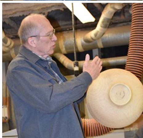
Ted showed a Cutsall grinder used to texture. By holding at a 45 degree angle, you can get an all-over pattern. The color is from black Krylon.
