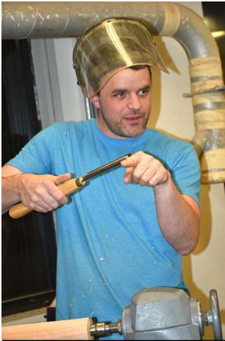
Showing how to start with the spindle roughing gouge.
