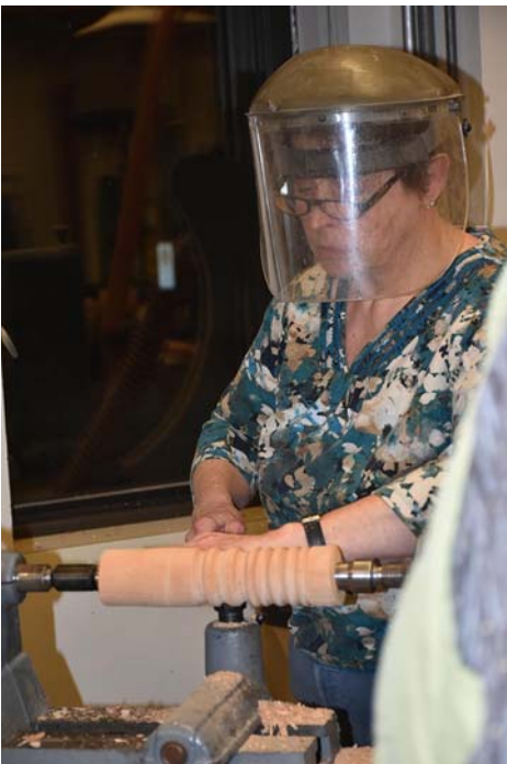
Showing how to start with the spindle roughing gouge.
