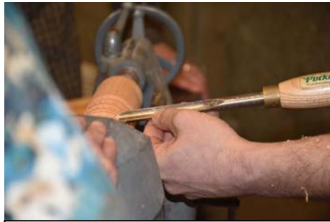
Rolling the spindle gouge to make even covers.
