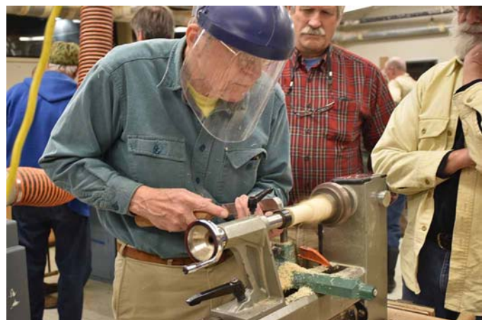
Ted shows the planning cut with the skew.
