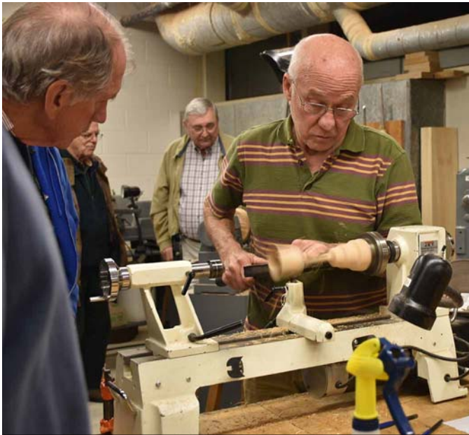
Russ demonstrates thin, offset turning on a goblet.
