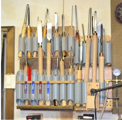
A tool rack of PVC pipe. The angled cuts allow for quick return of the tools and instant draining of chips.
