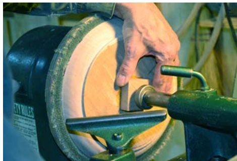
7. Ted uses a carpet-covered plywood plate as a jam chuck.
