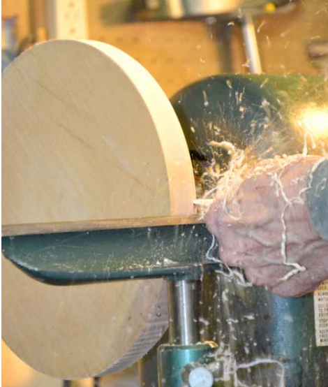
1. Ted trues the rim, working from the back side to minimize tear-out.
