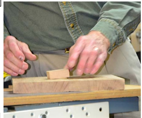
Ted glues a square block of hardwood on the base as a tenon for turning. It is centered to give maximum diameter of the platter from the board.
