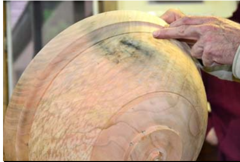
Russ shows a large black-cherry bowl with an ugly black stain caused by a metal hook in the wood.
