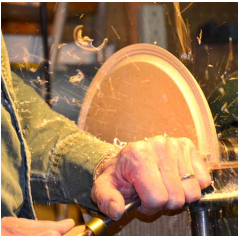
4. Starting to dig out the plate's surface.
