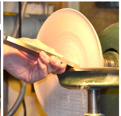
6. Using a massive scraper at a steep angle to even out the plate's surface.
