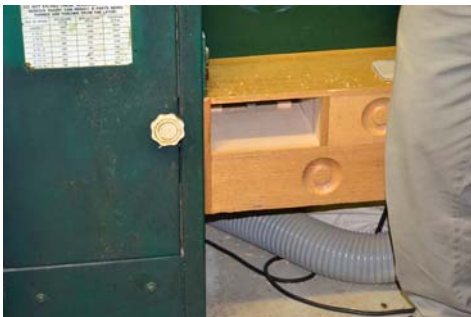
One of several drawer sets in Ted's shop. The recessed knobs keep from tangling power cords.
