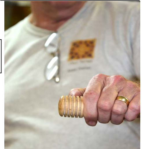
Mike Perron shows a honey dipper turned with a 'fluted' parting tool that avoids tear-outs, a bottle stopper/corkscrew, and a strong and reasonable screw chuck .
