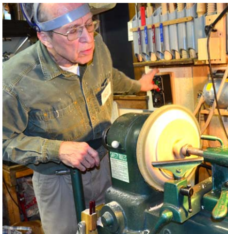
8. Centering up the platter before cutting the foot and the back side. All but the very center can be refined without moving the tail stock.
