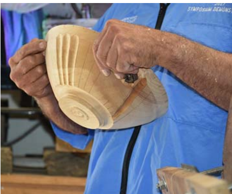
With careful use of the air hammer, very little sanding is needed to finish off.
