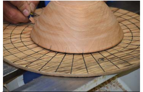
Al uses his jig to mark the rim of the bowl. As this is a smaller bowl, he uses every other mark on the jig to make wider grooves.
