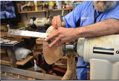
To demonstrate slanted flutes, Al marked the bottom of each flute but uses a flexible steel rule to draw guide lines. Instead of drawing a vertical line, Al goes from a bottom mark to a top mark one over from the bottom mark.
