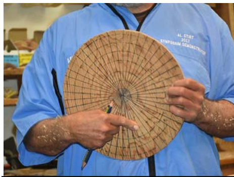
Using proper tools, Al made a jig with evenly spaced spokes and radius guides for marking blanks.
