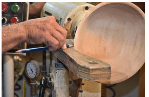
Another of Al's shop-made jigs. It's a wooden plane, heavy enough to prevent bending. It's curved to get close to the curve of a bowl and mounted on a section of pipe to ride on the banjo tool mount. The jig is set so the carpenter's pencil is exactly at the centerline of the lathe. Al draws a line from bottom to rim to guide for vertical flutes.
