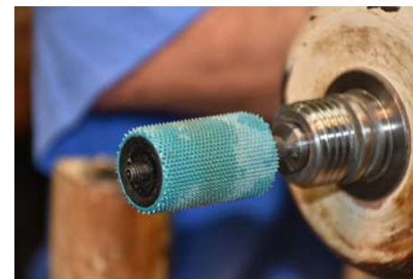
This is a coarse carbide grinding sleeve. Al gets good control for this method of fluting by mounting the tool in the lathe.
