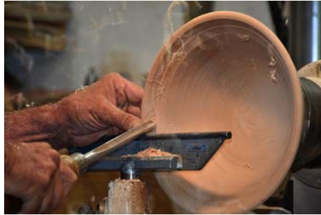
The bowl is getting near the right thickness. Al's left hand is steadying the bowl to smooth the cut.
