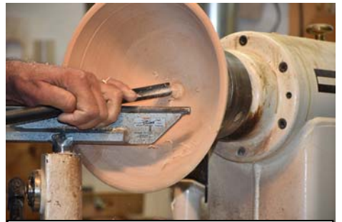
The interior is now quite smooth and the bowl thickness about right so the grooves have enough depth without breaking through.
