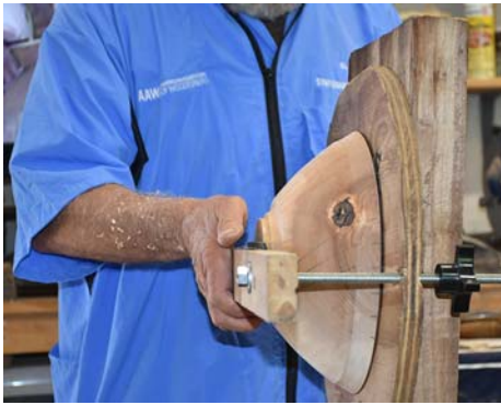
This is a heavy-duty clamp Al made up. Threaded rod and nuts to fit are easy to buy at a hardware store.
