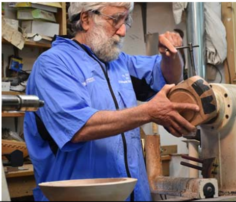
Al uses a jam chuck and the tail stock to mount a bowl blank. By having 4", 5", 6", and other size jam chucks, Al can quickly and securely mount once-turned blanks for further work.
