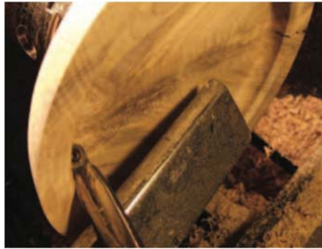
Figure 1. Undercutting the rim with the 1/2" Hunter Carbide Tool
