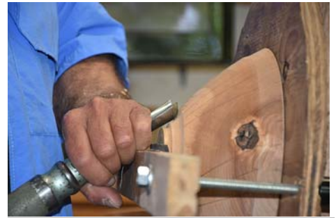
For this part of the demo, Al uses a Trow & Holden air hammer and modified #9 Swiss sweep gouge. Al's air hammer is modified with a variable air valve to control the action.
